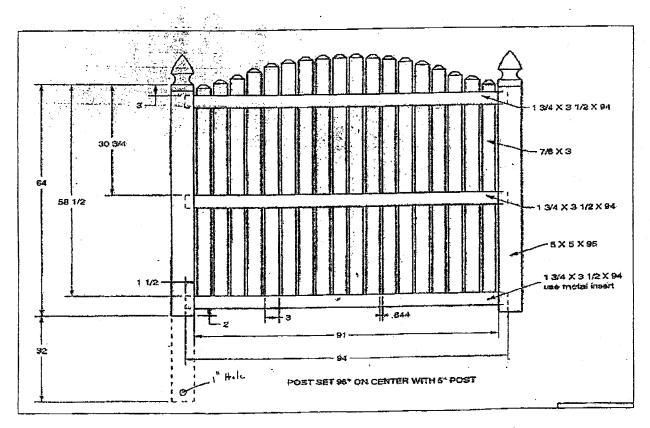
WHITE VINYL FENCE DETAIL SCALLOP OVER 72" WITH 1" SPACING 8' WIDTH
